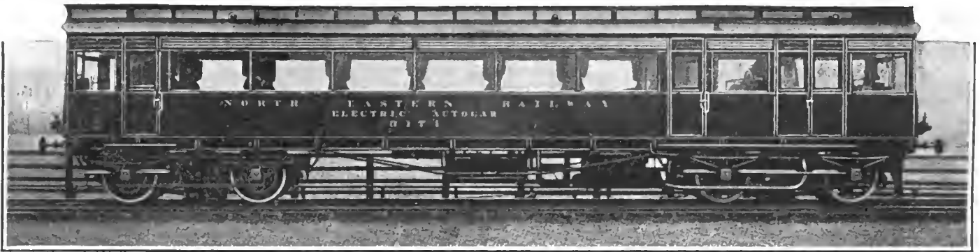
GASOLINE-ELECTRIC RAILROAD MOTOR CAR, EQUIPPED BY WOLSELEY FIRM FOR THE NORTH EASTERN RAILWAY OF ENGLAND.
